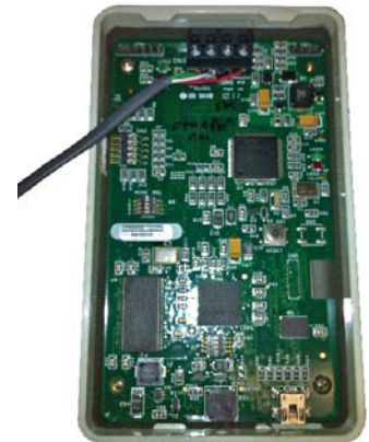
Fig 3. Interface connected to 4-pin header at top of display module.
