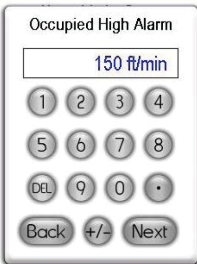
Fig 8. Enter high alarm setpoint for occupied mode using popup keyboard.
