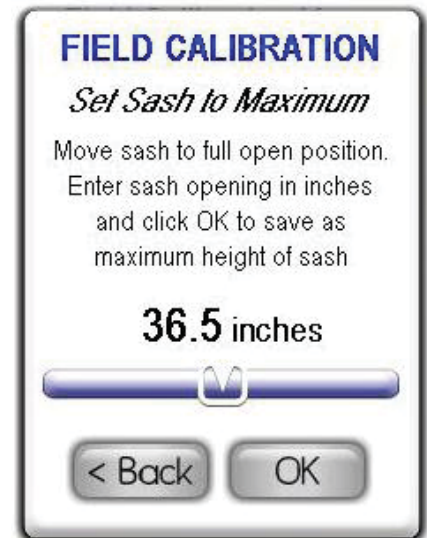
Fig 7. Set sash to maximum position and enter the height to complete the calibration procedure.
