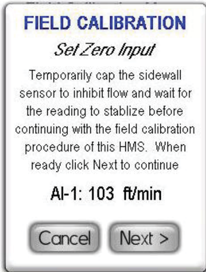
Fig 4. Sidewall sensor must be recalibrated once installed at the monitored fume hood.
