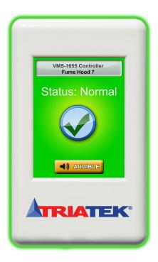
The VMS-1655M Fume Hood Monitor measures and controls the vortex pressure and adjusts to maintain proper fume hood containment. The VMS-1655M adjusts for environmental and usage conditions such as sash movement, fume hood loading, room pressure fluctuations, and cross drafts with active vortex stabilization in real time. Its alarm function notifies the user if the fume hood performance is compromised. Some of the features and benefits include:
